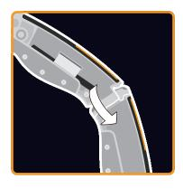
3. Unfold knife handle completely.
